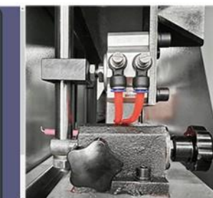
Abrasive belt pneumatic correction device
